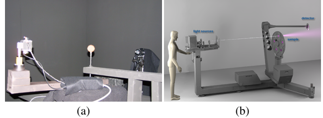
Figure 1: (a) A photograph of Matusik et al.'s BRDF measurement device [2003], (b) An overview of the pgII goniophotometer [Apian-Bennewitz 2014] (images from [Matusik et al. 2003; Apian-Bennewitz 2014]).
