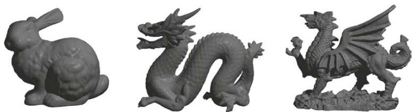
Figure 11. Bunny (69K primitives, 77 FPS), Stanford Dragon (871K primitives, 23 FPS) and Welsh Dragon (2M primitives, 18 FPS) ray traced in real time with full tree reconstruction on each frame using our Radix Sort algorithm.
