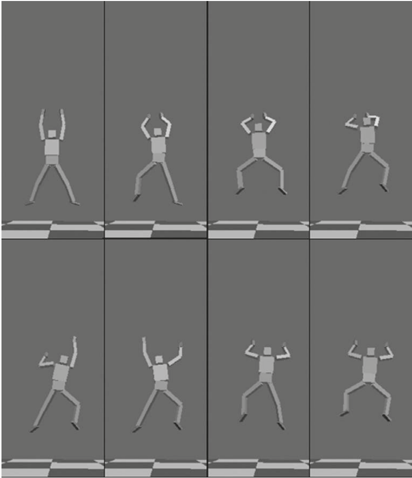
Asynchronized frog like climbing strategy. Asynchronized version of frog like strategy in Fig. 9. Asynchronization is achieved by altering swing wait durations. Swing wait duration of left arm and left leg is 0.5 and swing wait duration of right arm and right leg is 0.05.
